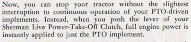
When your machine starts to choke up you simply push the PTO clutch lever-the tractor stops but the PTO driven implement goes right on working with full power. When it clears itself you let up on the clutch lever and move on again. Combines, Forage Harvesters, Corn Pickers, Manure Spreaders, Mowers, in fact every PTO driven implement you own, or plan to own, will do more and better work for you when you have Sherman Live PTO action in your tractor.
